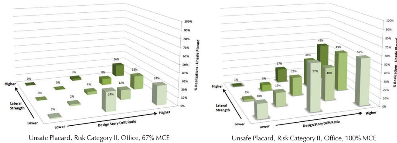
Figure 5-11 Probability of incurring an unsafe placard for 13 lateral strength/design story drift ratio combinations, Special RCSW, Risk Category II, office occupancies, 67% MCE and 100% MCE.
