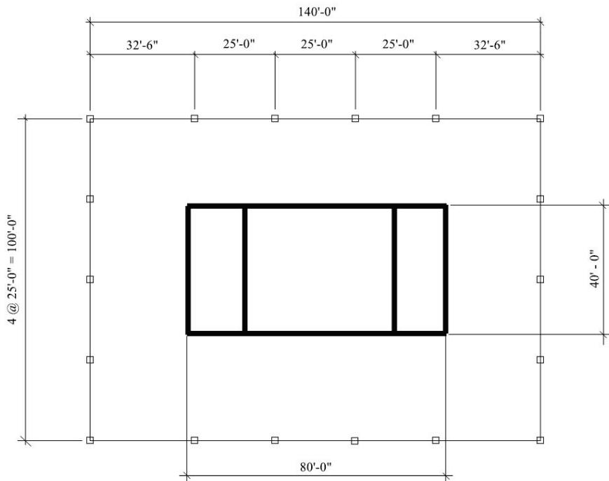
Figure 2-3      Typical plan for special reinforced concrete shear wall (SRCSW) archetypes.
