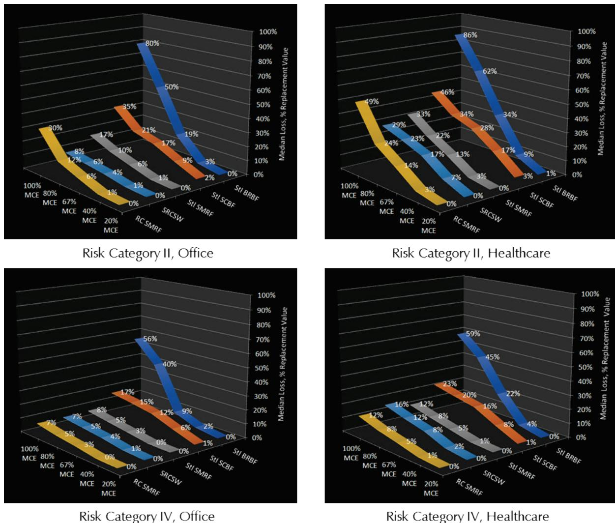
Figure 5-12 Comparison of median repair costs for each system, separated by Risk Category and occupancy, average of representative designs.
