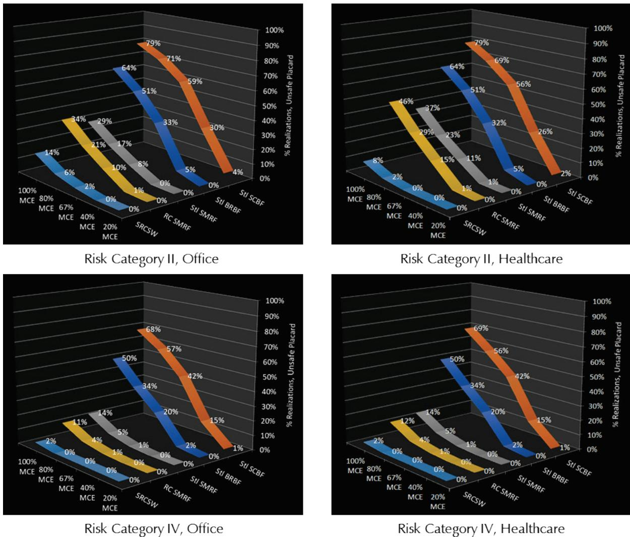
Figure 5-15 Comparison of median probabilities of incurring an unsafe placard for each system, separated by Risk Category and occupancy, average of representative designs.
