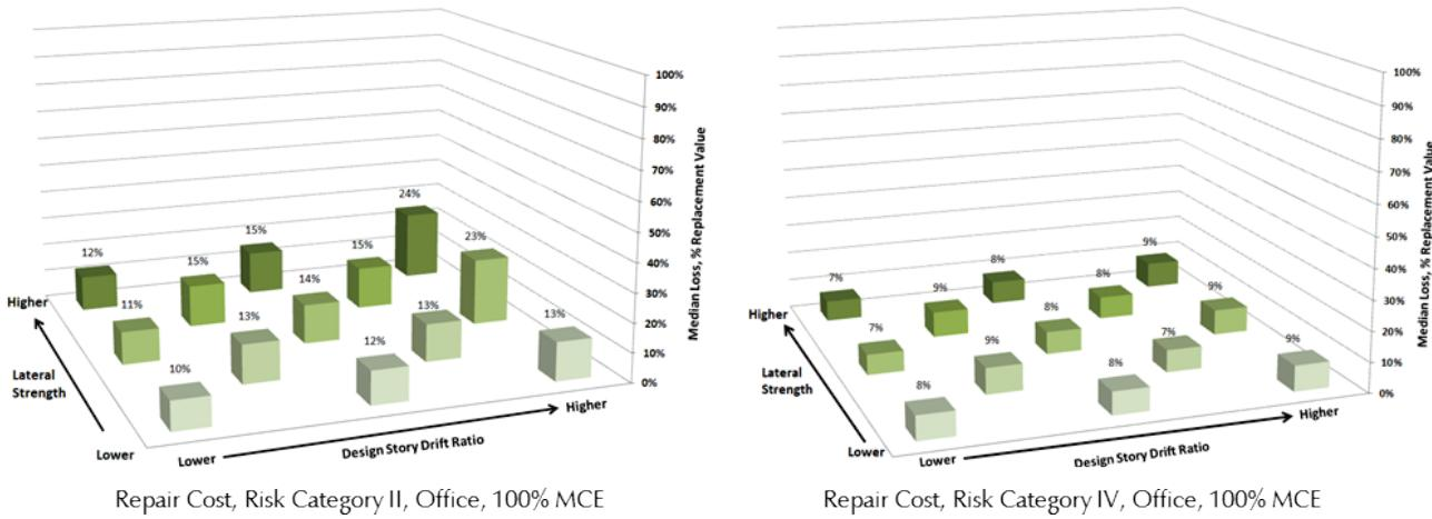
Figure 5-1 Median repair costs for 13 lateral strength/design story drift ratio combinations, Steel SMRF, Risk Category II and IV, office occupancies, 100% MCE.
