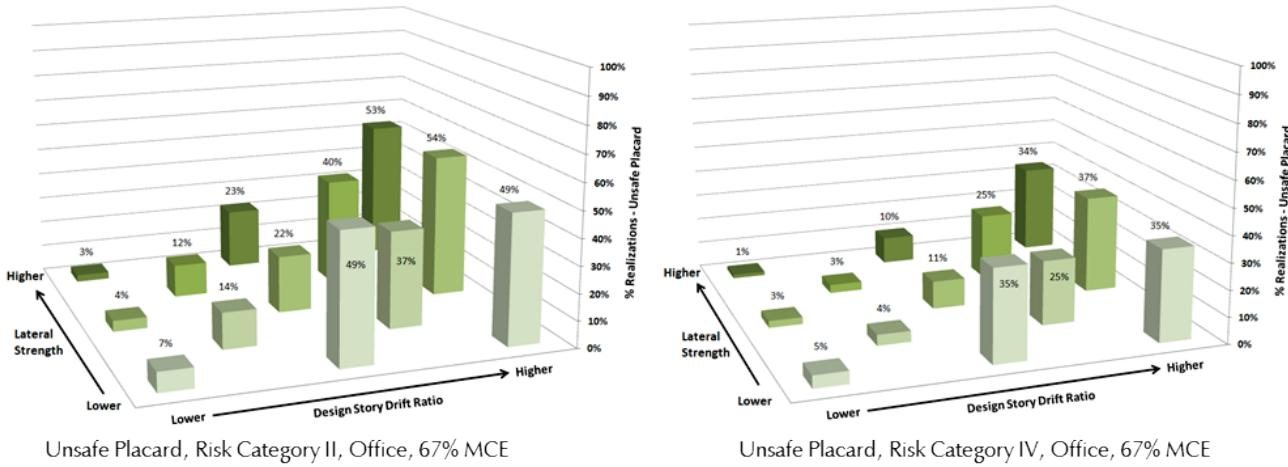
Figure 5-6 Probability of incurring an unsafe placard for 13 lateral strength/design story drift ratio combinations, Steel BRBF, Risk Category II and IV, office occupancies, 67% MCE.
