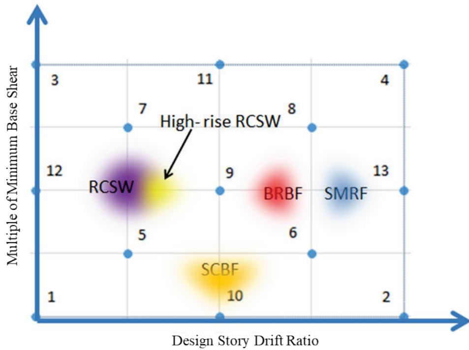
Figure 2-6 Plot of representative design points for each seismic force-resisting system in a generic design space.
