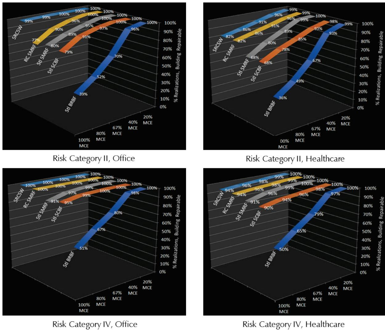
Figure 5-16 Comparison of median repairability for each system, separated by Risk Category and occupancy, average of representative designs.
