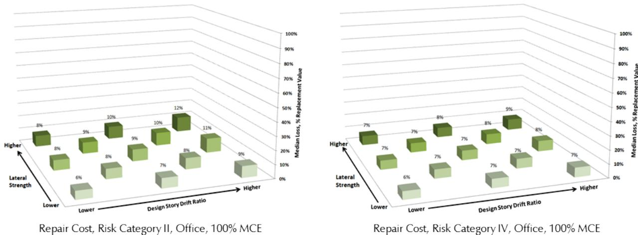
Figure 5-10 Median repair costs for 13 lateral strength/design story drift ratio combinations, Special RCSW, Risk Category II and IV, office occupancies, 100% MCE.
