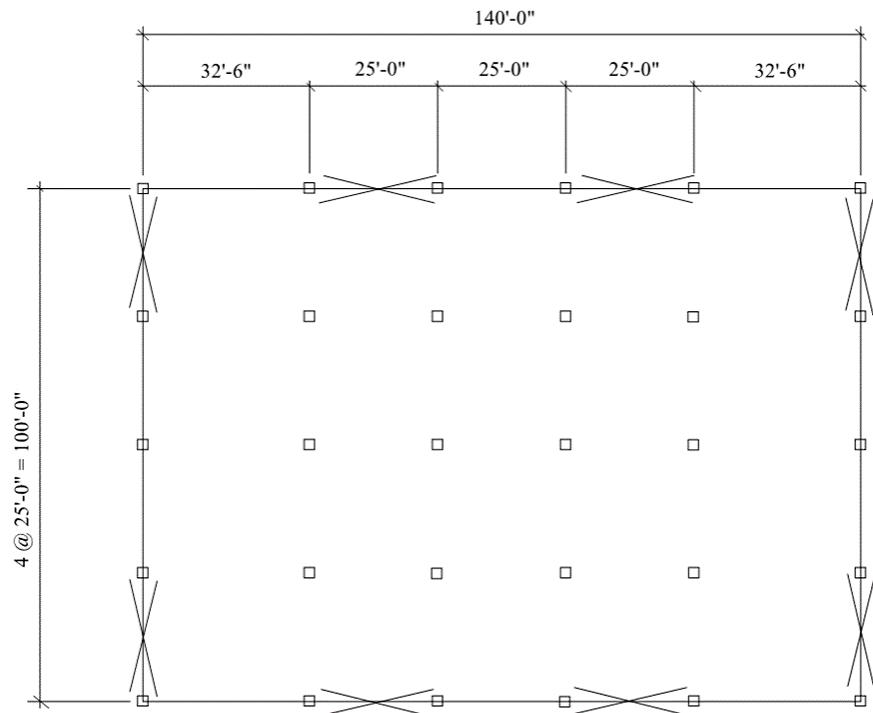
Figure 2-2      Typical plan for steel buckling-restrained braced frame (BRBF) and special concentrically braced frame (SCBF) archetypes.
