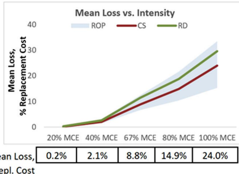
Figure C-3 Graph showing mean repair cost as a percentage of replacement cost on the User Interface tab.
