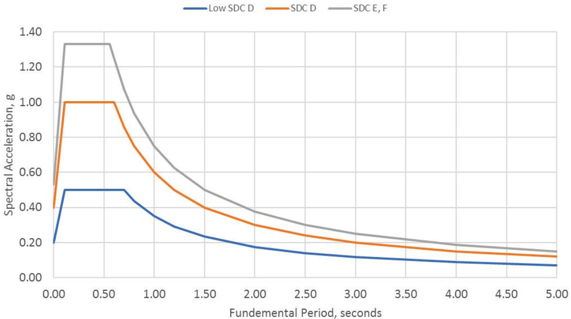
Figure 2-4      Design response spectra for sites corresponding to Low SDC D, SDC D, and SDC E/F hazard levels.
