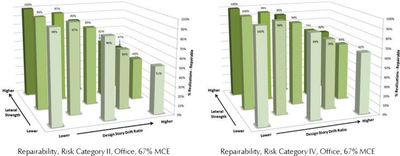
Figure 5-7 Repairability for 13 lateral strength/design story drift ratio combinations, Steel BRBF, Risk Category II and IV, office occupancies, 67% MCE.
