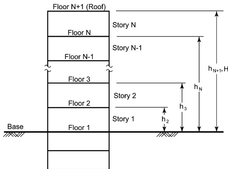
Figure 3-1      Definition of floor levels, story numbers, and floor heights used in the simplified analysis procedure (FEMA P-58, Volume 1).
