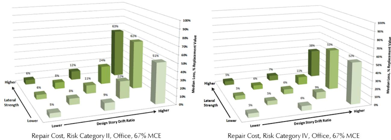
Figure 5-5 Median repair costs for 13 lateral strength/design story drift ratio combinations, Steel BRBF, Risk Category II and IV, office occupancies, 67% MCE.
