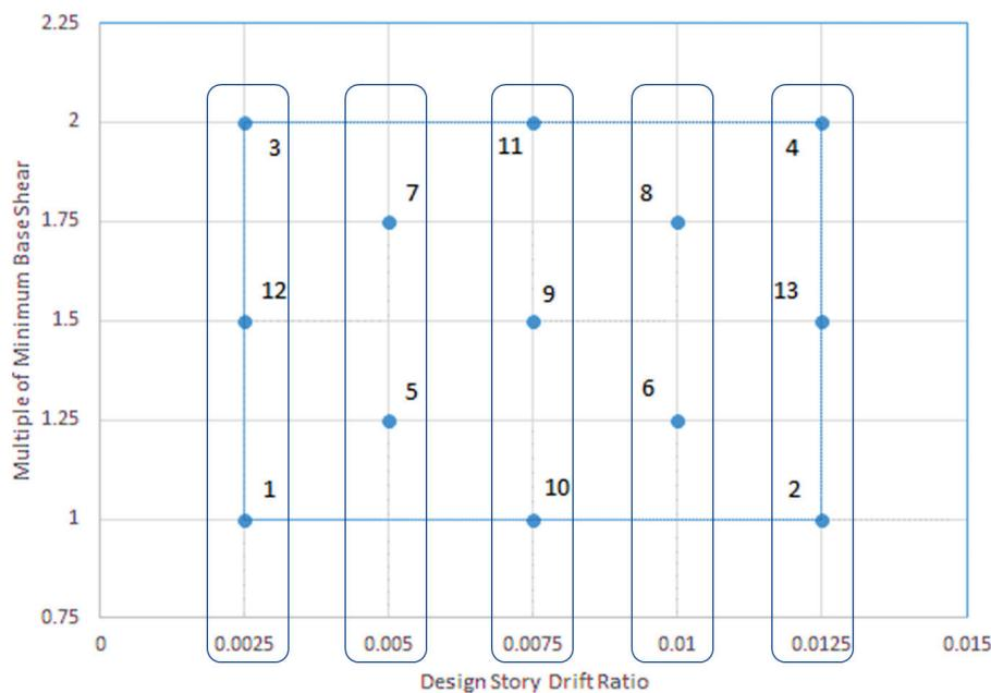
Figure 4-1 Design space for mid-rise, Steel SCBF, Risk Category II archetype, showing drift levels for displacement-controlled nonstructural component fragilities.
