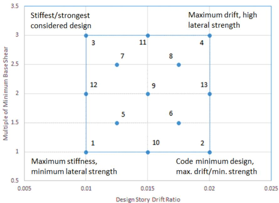
Figure 2-5      Typical design space showing 13 points used to characterize different strength and stiffness combinations for each archetype.
