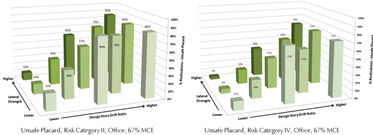
Figure 5-9      Probability of incurring an unsafe placard for 13 lateral strength/design story drift ratio combinations, Steel SCBF, Risk Category II and IV, office occupancies, 67% MCE.
