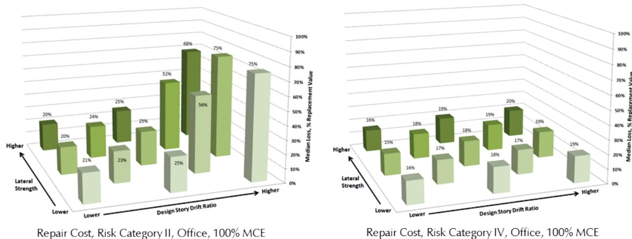
Figure 5-8 Median repair costs for 13 lateral strength/design story drift ratio combinations, Steel SCBF, Risk Category II and IV, office occupancies, 100% MCE.
