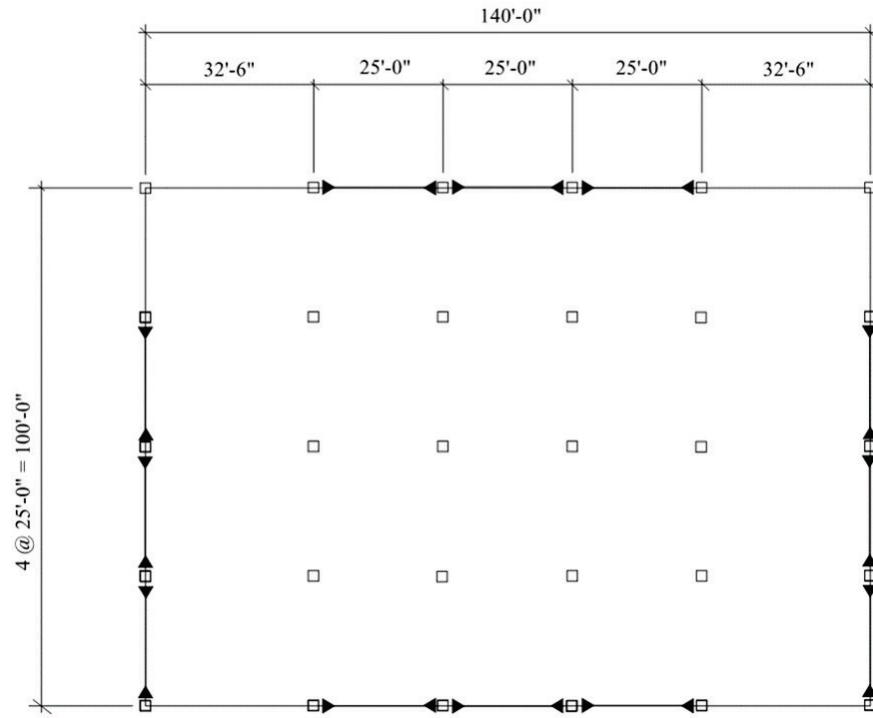
Figure 2-1      Typical plan for steel and reinforced concrete special moment-resisting frame (SMRF) archetypes.
