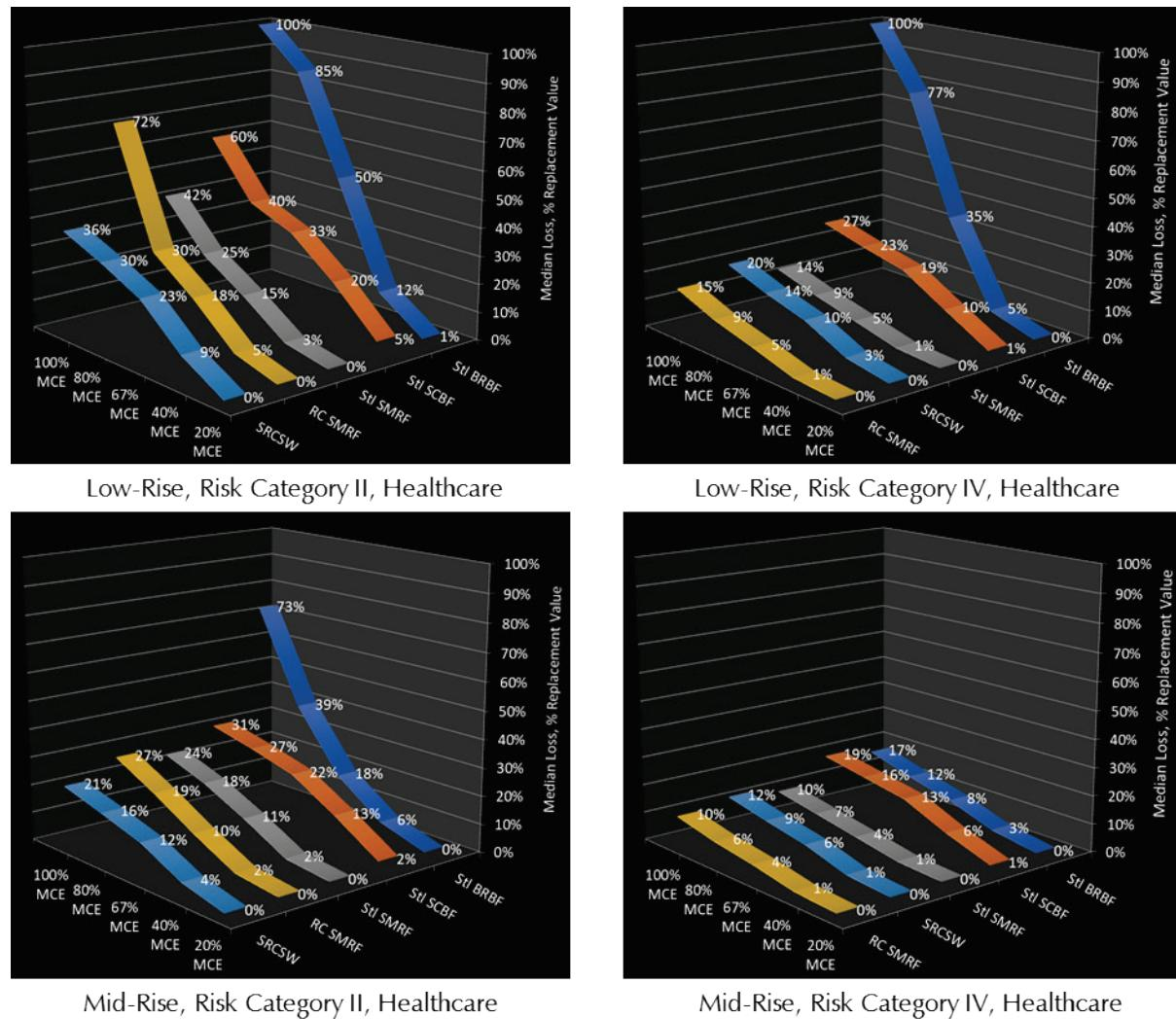
Figure 5-21 Comparison of median repair costs for healthcare occupancies, separated by building height and Risk Category, average of representative designs.
