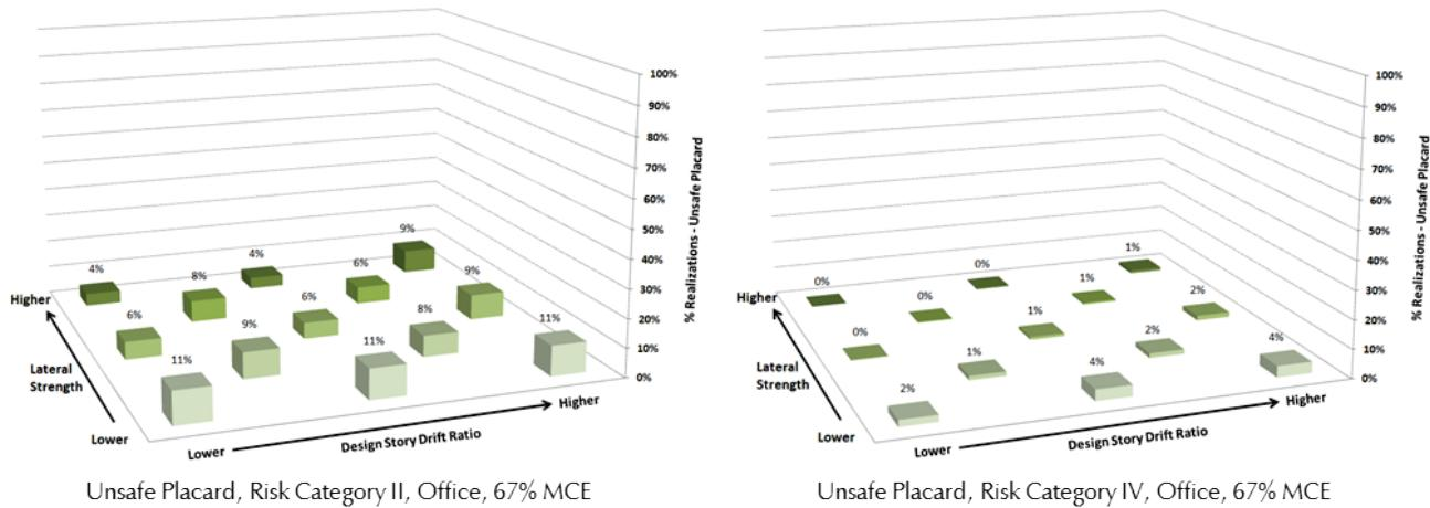
Figure 5-2 Probability of incurring an unsafe placard for 13 lateral strength/design story drift ratio combinations, Steel SMRF, Risk Category II and IV, office occupancies, 67% MCE.
