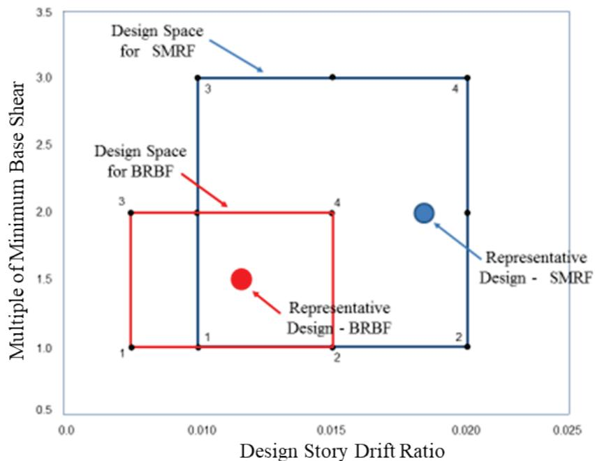
Figure 2-7 Comparison of design space limits and representative design points for mid-rise, Risk Category II, Steel SMRF and BRBF archetypes.
