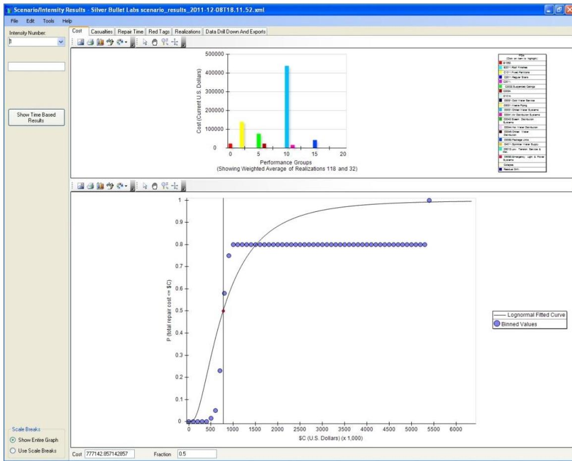
Figure 4-4 Sample PACT output for replacement costs associated with a scenario- or intensity-based assessment (FEMA, 2012b).
