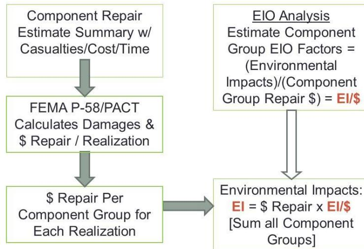
Figure 6-3 Flowchart of EIO Procedure 1B, Realization-Based Approach.
