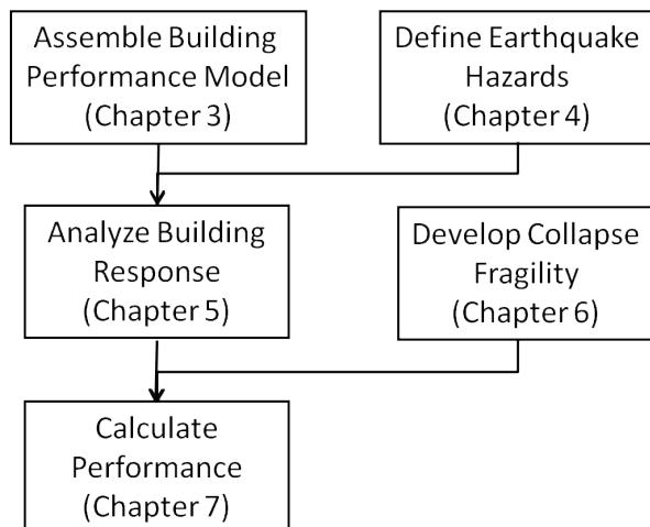
Figure 4-1 Flowchart of the FEMA P-58 methodology for seismic performance assessment of buildings (FEMA, 2012a).
