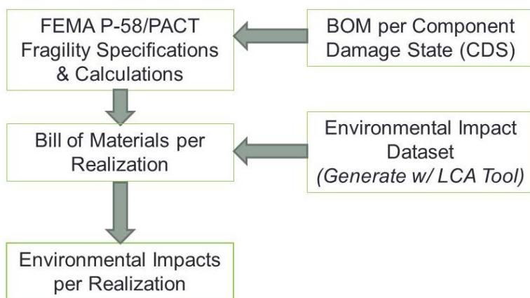
Figure 6-6 Flowchart of BOM Procedure 2B, Realization-Based Approach.
