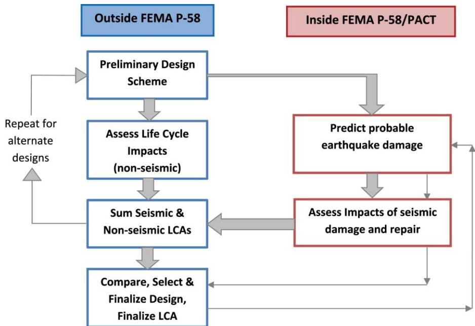
Figure 7-1 Flowchart of the sustainable seismic design process for new buildings.
