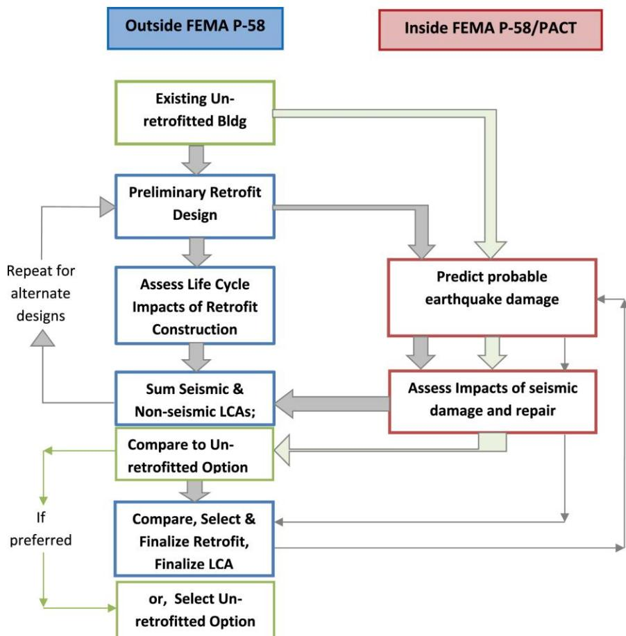
Figure 7-2 Flowchart of the sustainable design process for seismic retrofit.
