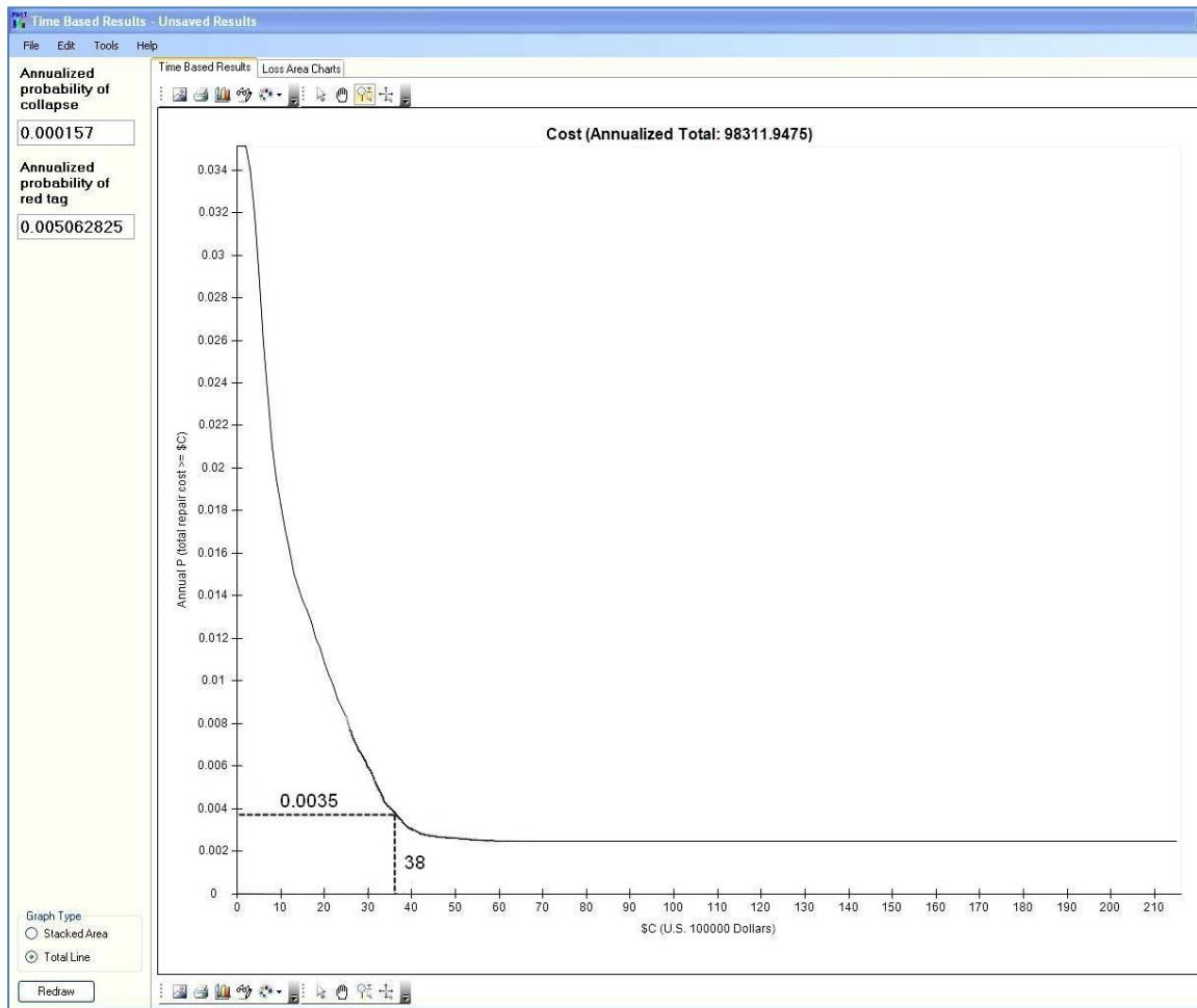
Figure 4-7      Sample PACT output showing annualized repair costs for a time-based assessment (FEMA, 2012b).
