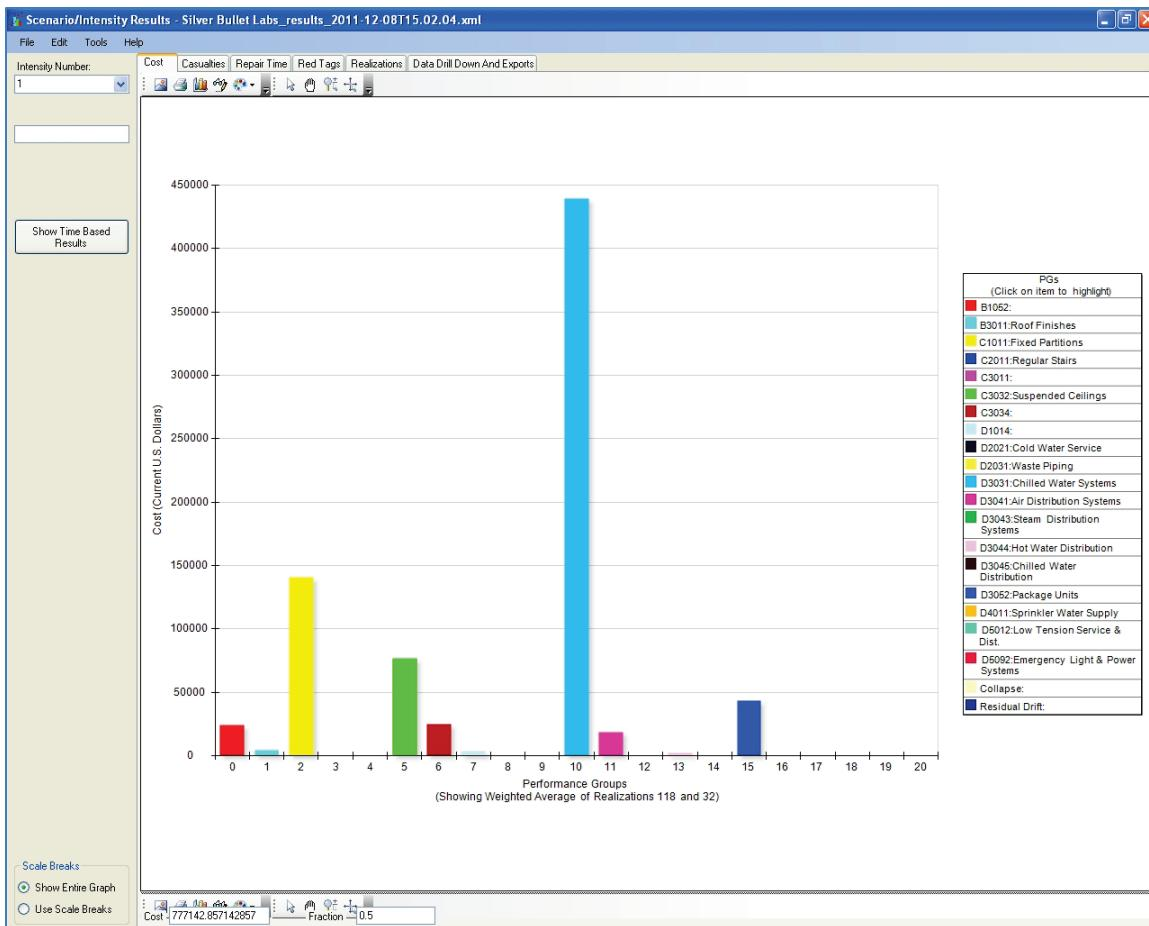
Figure 4-5      Sample PACT output showing repair cost by performance group (FEMA, 2012b).
