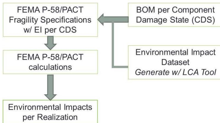
Figure 6-5 Flowchart of BOM Procedure 2A, Component-Based Approach.
