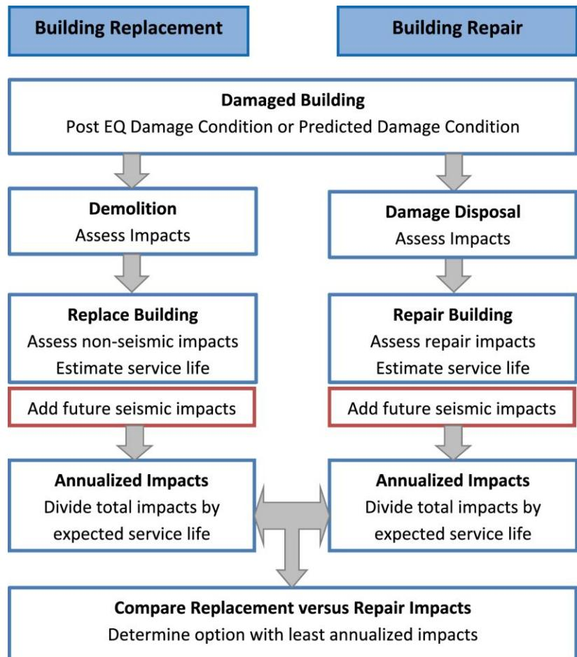
Figure 7-3 Flowchart for repair versus replacement decision making.
