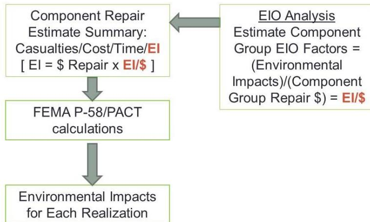
Figure 6-1 Flowchart of EIO Procedure 1A, Component-Based Approach.
